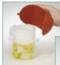
For secure handling and thermal protection
